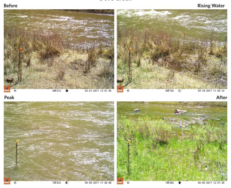
**Figure 4.** Dove Creek staff gage at pre-release, rising water, peak-release, and post-release. Notice river rising substantially out of its banks at peak-release but with very little change in the amount of woody vegetation.
