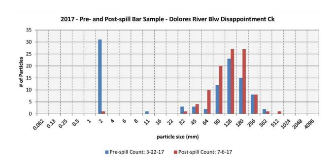
**Figure 2.** Slickrock Downstream (Below Disappointment Creek) site Wolman pebble count results 2017. These important results show that 2 mm particles were almost completely removed from the site.
