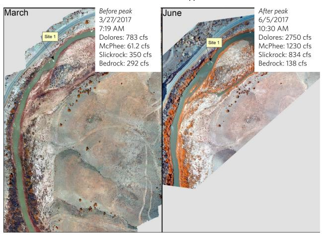
**Figure 7.** Drone imagery comparison March versus June 2017 at the Slickrock Downstream site. There is very little difference in planform pre- versus post-release. Most of the differences observed is because of higher water levels in June photos. Higher flow caused side-channel flow here, and floodplains stand out as a whiter color because of sand deposits.
